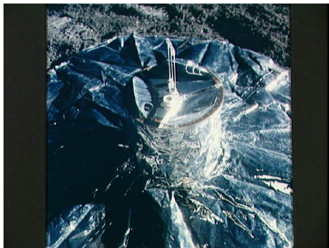
A close-up view of the Passive Seismic Experiment, a component of the Apollo Lunar Surface Experiments Package (ALSEP) which was deployed on the Moon by the Apollo 14 astronauts during their first extravehicular activity (EVA-1). (NASA/JSC)
