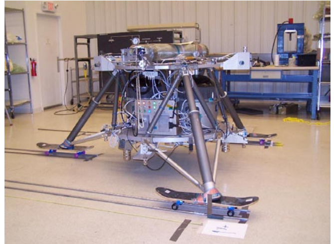
The robotic lander prototype was placed on modified skateboards and a customized track system as a low-cost solution to control movement during final testing of the prototype's sensors, onboard computer, and thrusters. Credit: NASA/TBE
