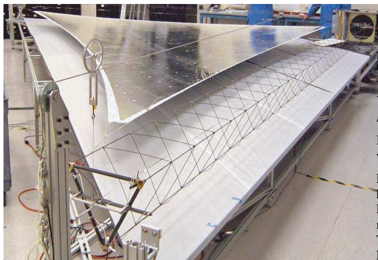
Caption: SAILMAST is the thin triangular truss in front of the picture. It is attached to a section of a silver foil solar sail section shown here in a laboratory test. The mast in the picture is 2m (6 ft) long. The Space Technology 8 mission will test the SAILMAST, which is 20 times longer.
